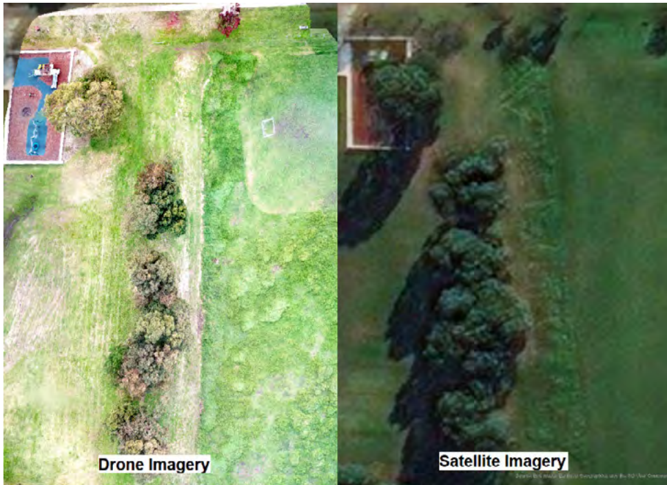
Image: Comparison of drone derived orthomosaic with satellite imagery at Lakelands oval.
