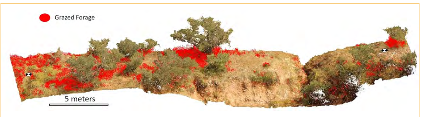
A comparison of a transect before and after grazing. The red shows regions of difference between the two 3D point clouds, indicating where grazing has occurred. Source: Jeff Gillan
